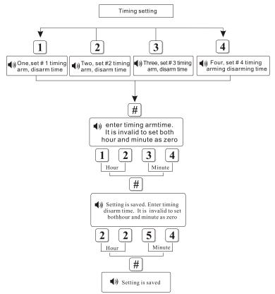
Example: Set timing arm at 6:50 AM, timing disarm at 8:35 PM.(Enable set total 4 groups of timing arm/disarm time)
