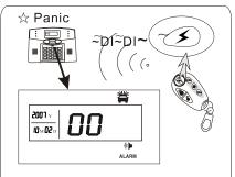
Press the panic button on remoter, or press "help/bypass" key on panel for 3 seconds, and 10seconds later the panel will dial the preset phone number. And you can disarm to cancel alarm.
