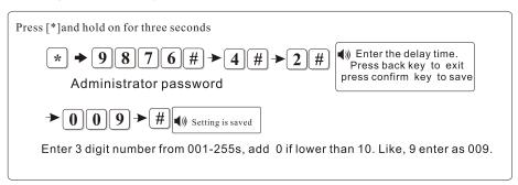
5.63 Exit delay setting: the period from user arm to the system armed successfully. This is for user's convenience to exit after arm operation. (default value is 10s)
