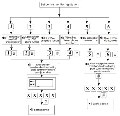
The user code in the CMS setting which is identification code in the CMS. And the user code in transfer alarm setting is user, identification code between same model panel
